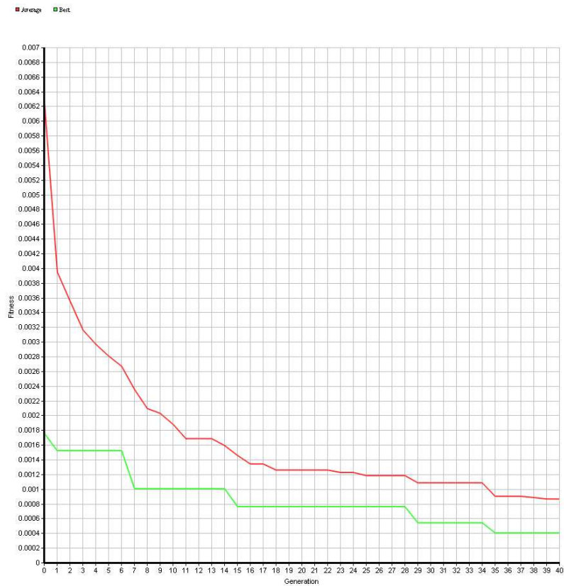
Fig. 7. Fitness progress of the parameter learning process. Best individual and average error in the population is shown.
